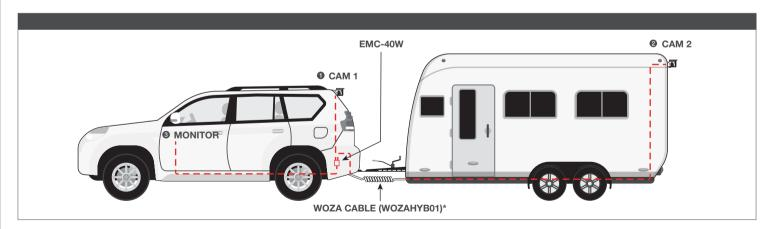
When no Woza Cable is connected, CAM 1 will be displayed on the monitor as normal.
