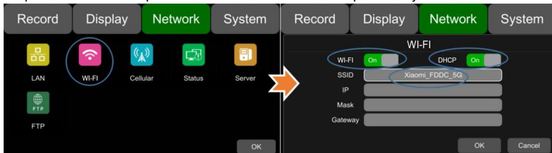
Step 4: Click SSID sub-menu and the WIFI hot spot shows up. Select which hot spot to connect and enter the password.
