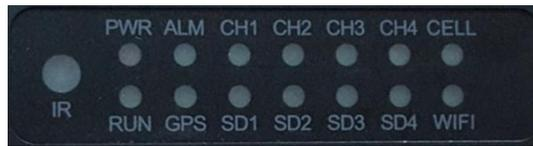
**PWR:** Red LED, lights up when DVR is powered on, and goes out when power is cut off.
