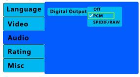
User can adjust S/PDIF terminal audio output by choosing number output set, to make it work harmony with other equipment(for example, receiver and sound box.
